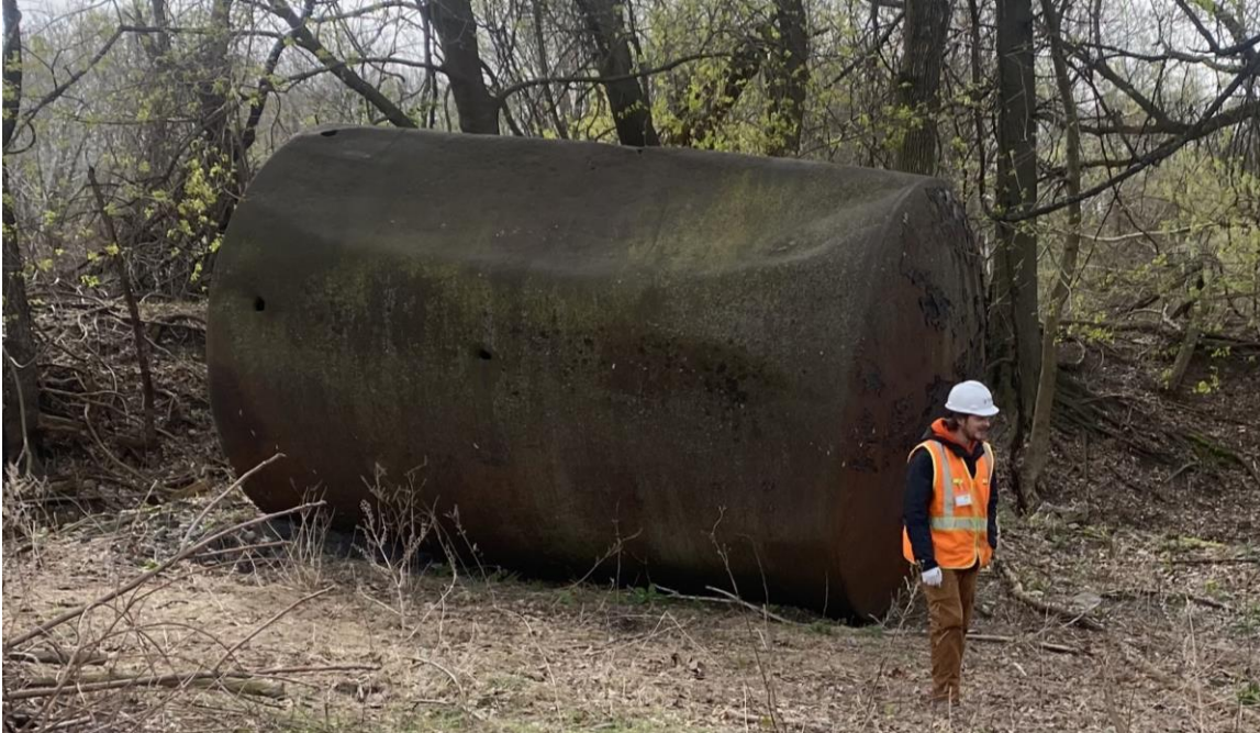
Underground Storage Tank
