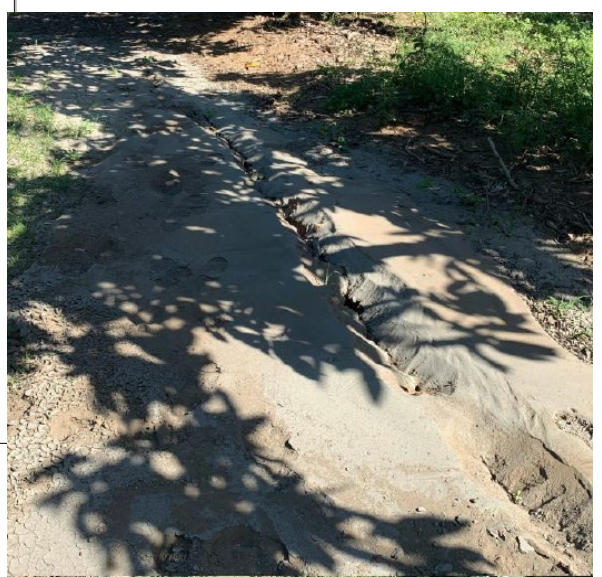
Sand ejecta, sand boils, lateral spreading Earthquakes January 7 Bernal et Al, 2020
